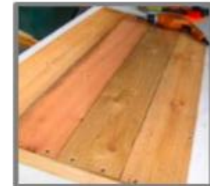
If you measured correctly the planks should be flush with the ribs and rails.
